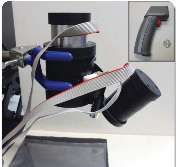
A bench-top scanner detects oxygen levels within sealed food packages.
